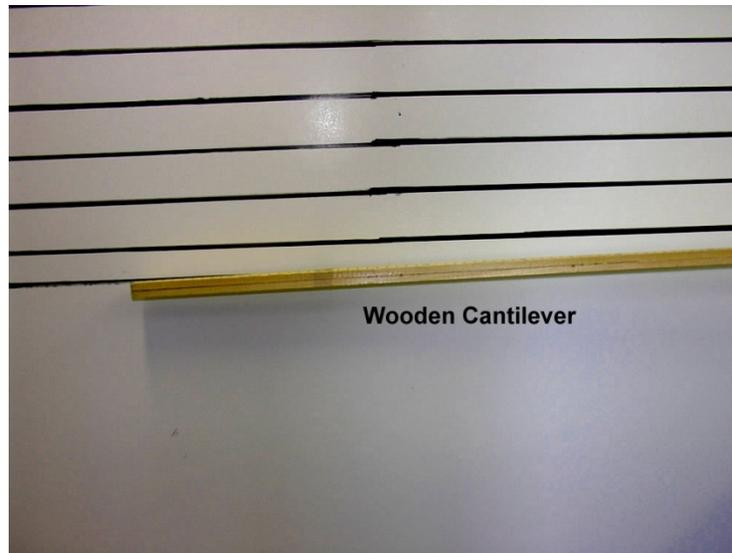
*Cantilever in front of white board with reference lines. This activity can be done with any type of individual planks or sticks. The equations apply to any cantilever structure that has a rectangular cross section of thickness,  $t$ , width,  $w$  and length,  $l$ .*
