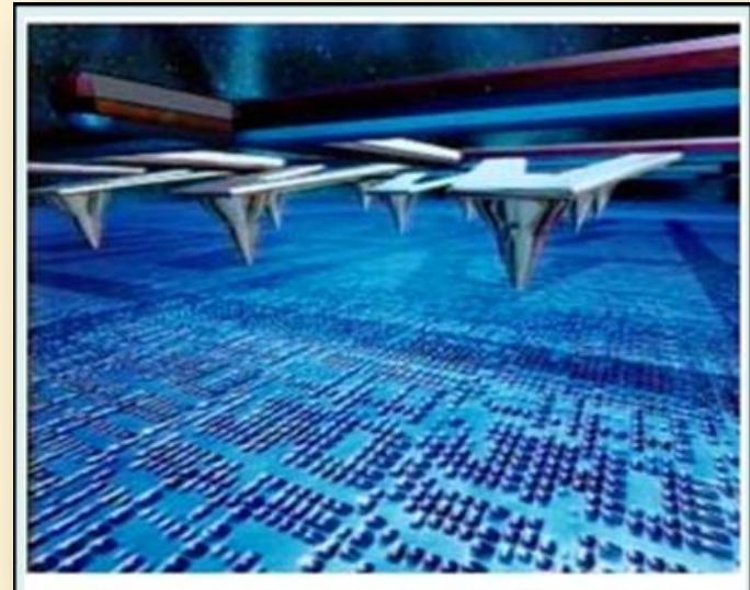
Cantilever Array for Read/Write Memory [Image courtesy of IBM]
