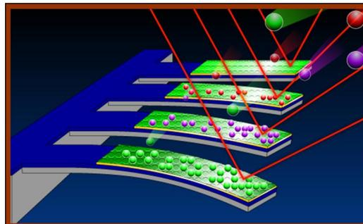
The amount of change in resistance and change in angular deflection is a measurement of how much target material is adsorbed.
