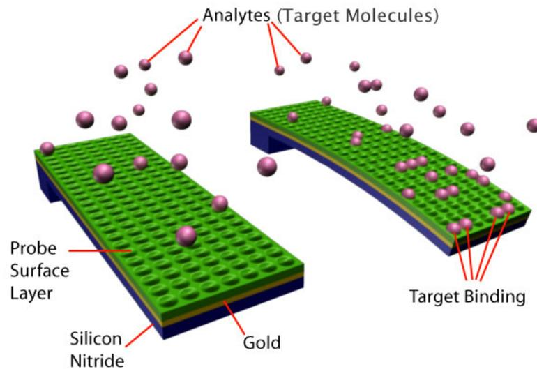
*Surface Reaction between Analytes and Probe Coating Molecules*
