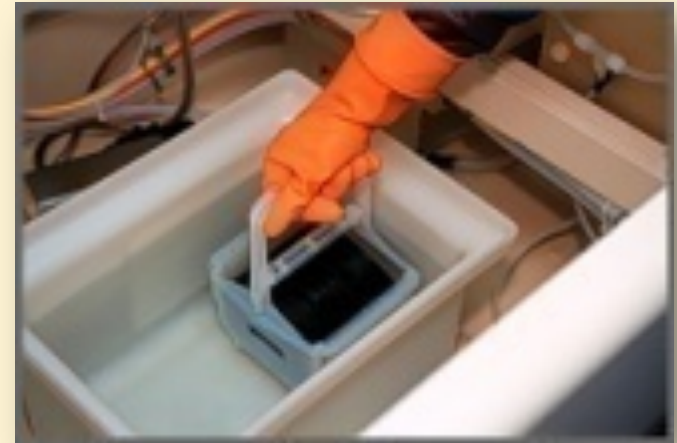
Wafer Carrier in Etchant Solution [Photo courtesy of Bob Willis]
