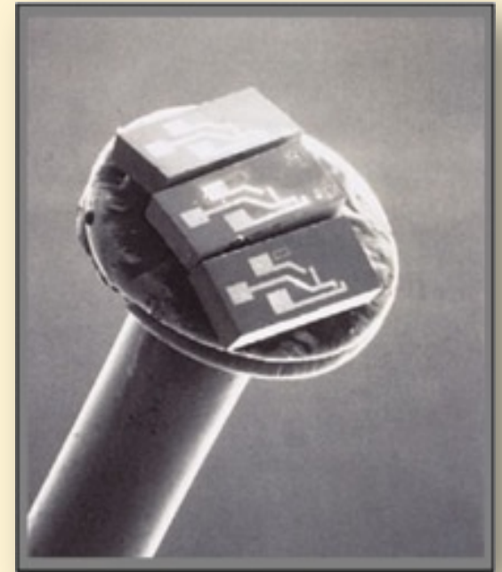
MEMS Blood Pressure Sensors on the head of a pin. [Photo courtesy of Lucas NovaSensor, Fremont, CA]
