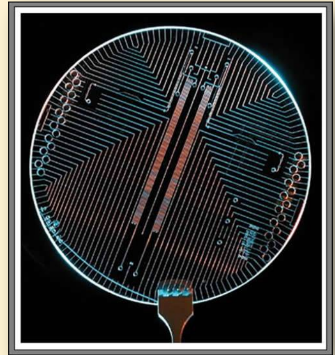
Lab-on-a-Chip (LOC) [Printed with permission. From Blazej, R.G., Kumaresan, P. and Mathies, R.A. PNAS 103,7240-7245 (2006)]
