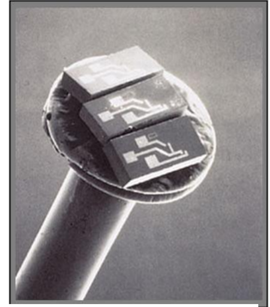
MEMS Blood Pressure Sensors Photo courtesy of Lucas NovaSensor, Fremont, CA]
