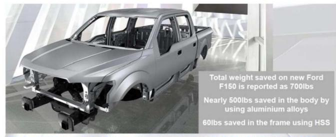
The Ford F150 truck is the first high volume application of LWV technology in the USA
