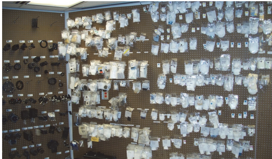
Figure 5 Peg-board storage of optical components
