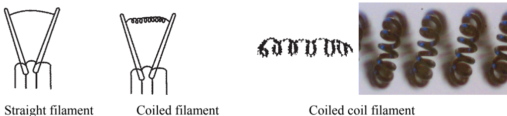
Figure 3-5 Types of incandescent filaments. Filaments are arranged upon support structures within the bulb in a variety of ways. The filament itself may be either, straight, coiled, or coiled coil.
