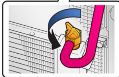
Air bleed valve on top of dedicated radiator
