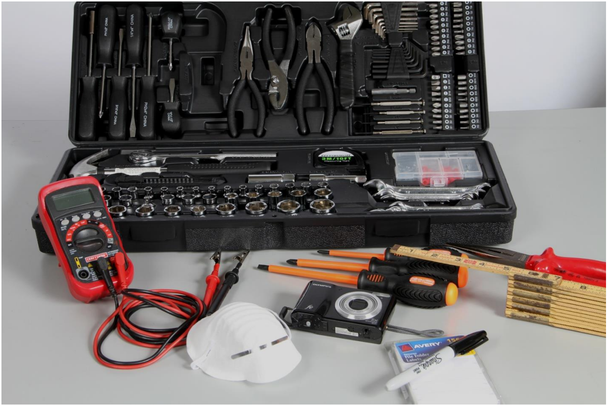
Standard Tools with Insulated Tools in Foreground
