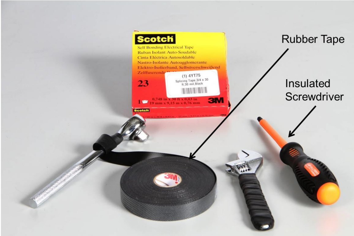
Standard Tools with Insulated Tools in Foreground
