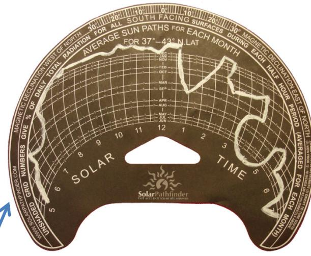
To find the site percent, add the numbers in the unshaded part of the sunpath arc. The site tracing shown here has 64% solar available for January, found by adding  $2 + 3 + 4 + 5 + 6 + 7 + 7 + 8 + 8 + 8 + 6 = 64\%$ . This shows that only 64% of the potential available radiation is reaching this particular location during January. 36% of the potential available radiation is blocked out in the middle of the winter.
