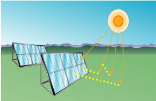
Flat-plate collectors, which typically contain a large number of solar cells mounted on a rigid, flat surface, can make use of both direct sunlight and the diffuse sunlight reflected from clouds, the ground, and nearby objects.
