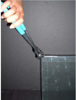
Figure 6- Place nippers on the glass corner & pinch! Figure 7- Study and discuss the fracture.
