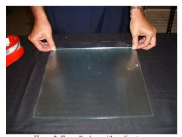
Figure 2- Tape all edges with sealing tape.
