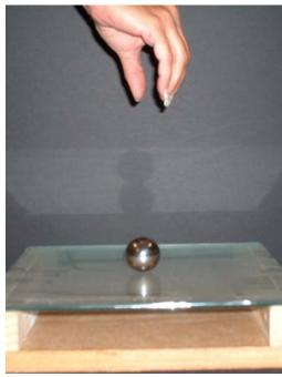
Figure 5- Drop the ball on to the center.
