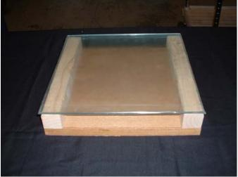
Figure 3- Place the wrapped glass pane on the wood blocks.
