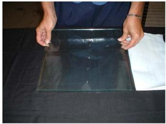
Figure 1- Peel contact paper and wrap glass pane.
