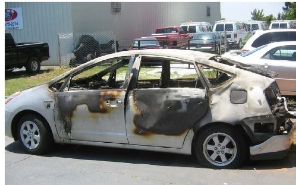
Figure 1--Fire Damaged PHEV Prius
