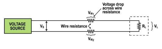
$$V_L = V_S - V_{W_1} - V_{W_2}$$
