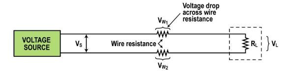
$$V_L = V_S - V_{W_1} - V_{W_2}$$
