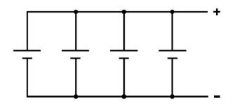
Parallel connection increases cell current capacity
