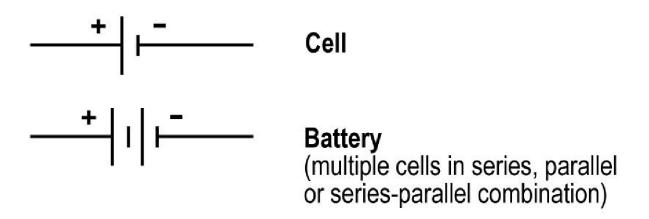
As stated earlier, cells consist of a cathode, an anode, and an electrolyte. The figure above shows the schematic symbols of a cell and battery.
