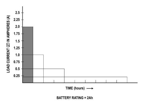
Ampere-hour rating (or capacity) is used to indicate the capacity of a cell. It is the maximum available current supplied over time. The ampere-hour rating of a battery is the amperes (A) drawn over some time usually hours (h). Ampere-hours = Ah.
