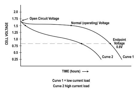
The amount the battery discharges for different current loads can be plotted showing the cell voltage and the time in hours.
