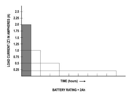
Batteries have an Ah rating such as 200 Ah. This means that the battery can supply 200 A for one hour until it is discharged.
