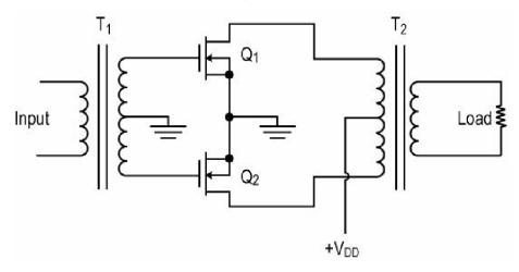
An older form of power amplifier is the transformer coupled push pull circuit. It was once widely used in audio amplifiers but has been replaced by the complementary symmetry circuit described earlier because no heavy and expensive transformers are needed.
