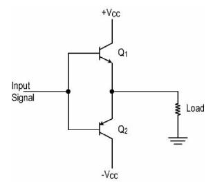
The circuit operates as a class B amplifier. The NPN transistor conducts on the positive half cycles and the PNP transistor conducts on the negative half cycles.
