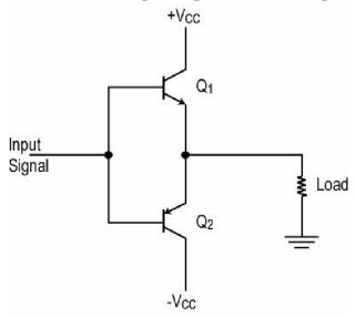
A complementary symmetry amplifier is a good illustration to show the characteristics and limitations of linear power amplifiers. It is used in over 90% of all linear power amplifier applications.
