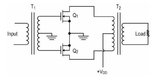
However, this circuit suffers from crossover distortion because  $Q_1$  and  $Q_2$  are enhancement mode MOSFETs that require a gate voltage higher than the threshold to conduct.
