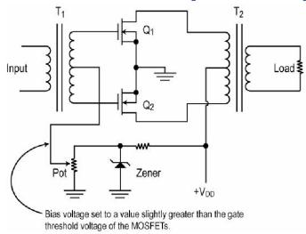
In this circuit, a Zener diode is biased into conduction and a pot is used to apply a bias voltage to the center tap of the secondary of  $T_1$ . This bias voltage appears at the gates of  $Q_1$  and  $Q_2$ .
