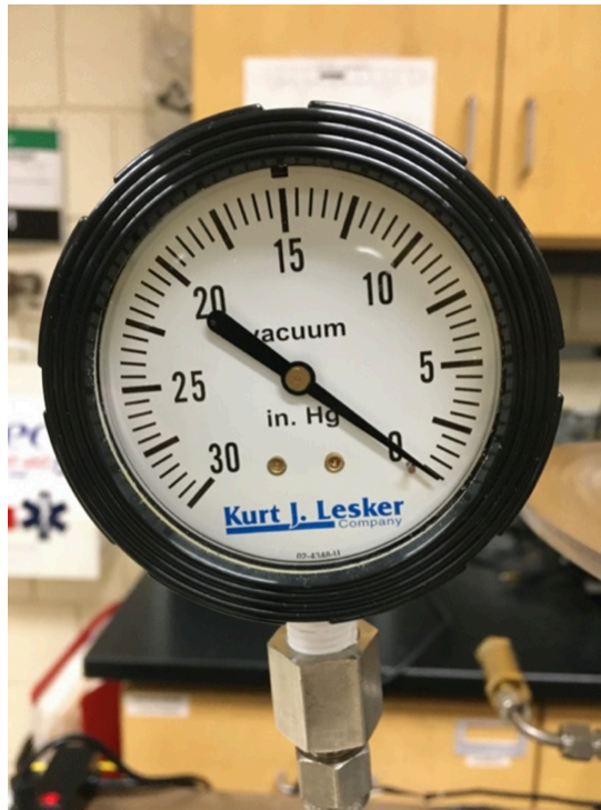
Figure 3.1. Bourdon gauge reading of atmospheric pressure. Photo is provided by Nancy Louwagie, Normandale Community College.
