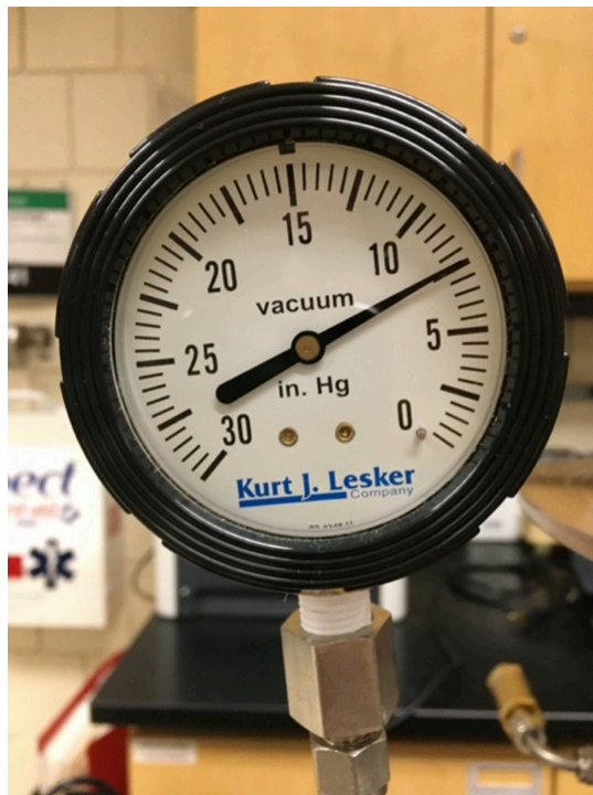
Figure 3.2. Bourdon gauge reading of below-atmospheric pressure. Figure provided by Nancy Louwagie, Normandale Community College.
