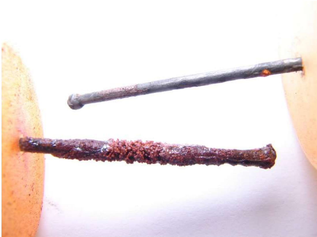
The top nail was exposed to DWSD water for one month. The bottom nail was exposed to Flint River water for one month. Credit: FlintWaterStudy.org
