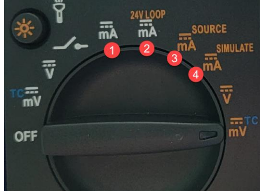
Signal generator dial setting should be on mA SIMULATE (4)
