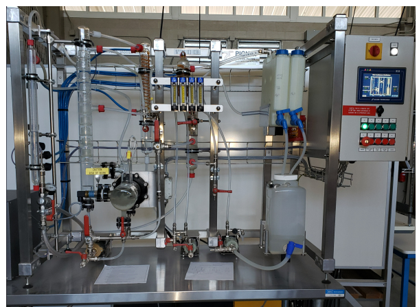
Distillation Training Unit
