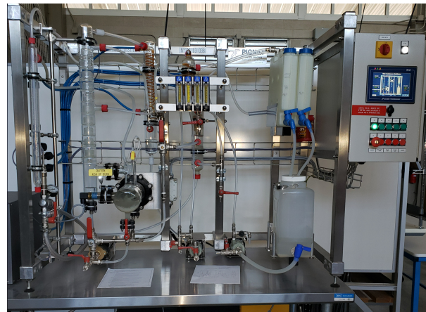
Distillation Training Unit
