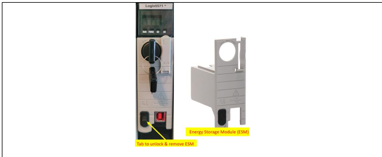
Figure 6. Removing the ESM from the controller.
