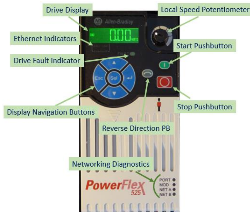
Figure 2. Identifying the devices on a PF525 VFD.
