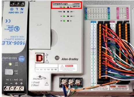
It is important to know the part number for the CompactLogix processor, especially when a new project is created in the Studio 5000 software, since this will also configure the I/O. The processor number should be on the front of the CompactLogix unit, or on the side of the processor module when working with a modular CompactLogix system. The technical manuals will also specify that the L27ERM-QBFC1B unit is part of the **5370 L2** family of processors.
