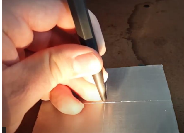
Figure 8. Center punch the scribe marks.
