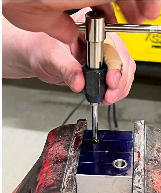
Figure 11. Hand tapping a thread on the NIMS workpiece.
