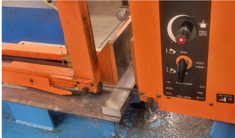
Figure 3. Sawing the block from a piece of stock.
