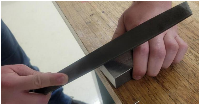
Figure 5. Removing sharp edges and burrs using a file.
