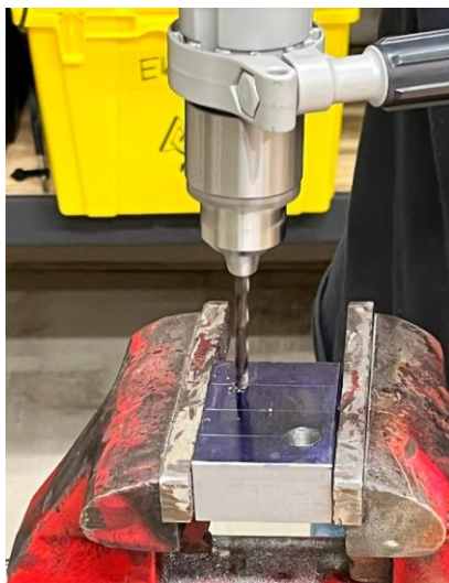
Figure 9. Drilling the holes in the workpiece.
