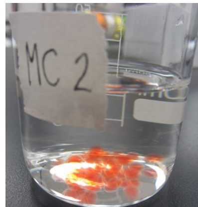
Figure 3: a) Approx. 25 uncoated alginate beads in 30mL DI water (MC1); b) Approx. 25 chitosan-coated alginate beads in 30mL DI water (MC2).
