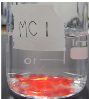
Figure 3: a) Approx. 25 uncoated alginate beads in 30mL DI water (MC1); b) Approx. 25 chitosan-coated alginate beads in 30mL DI water (MC2).
