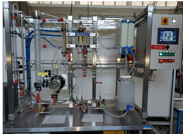
Distillation Training Unit
