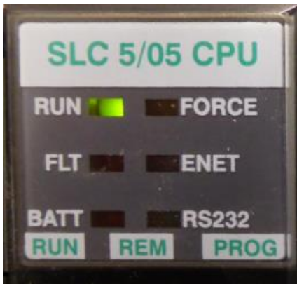
SLC-500 processor diagnostic indicators
