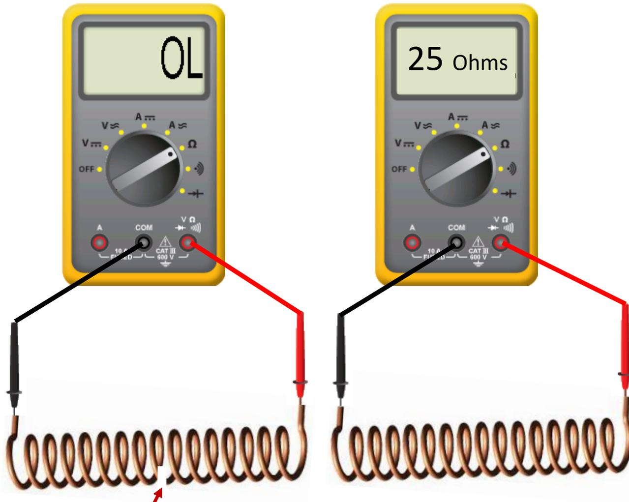
Coil is open, so it will display OL for Open Line
