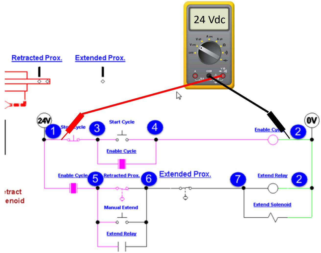
This slide will show the voltages that should be measured if both rungs are powered, and the solenoid is energized.
