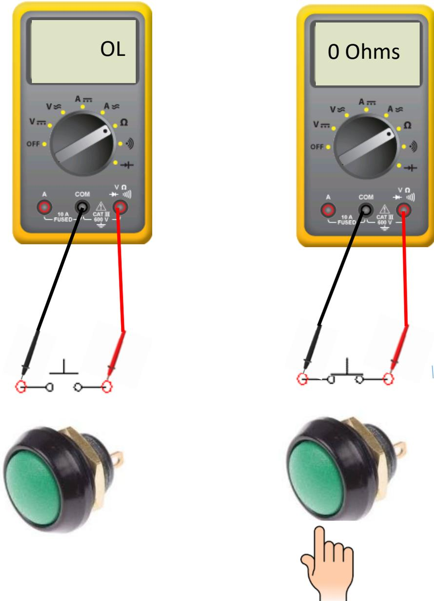
Many times a user must test a Normally-open pushbutton when it is out of the circuit, to determine if it is faulty.
