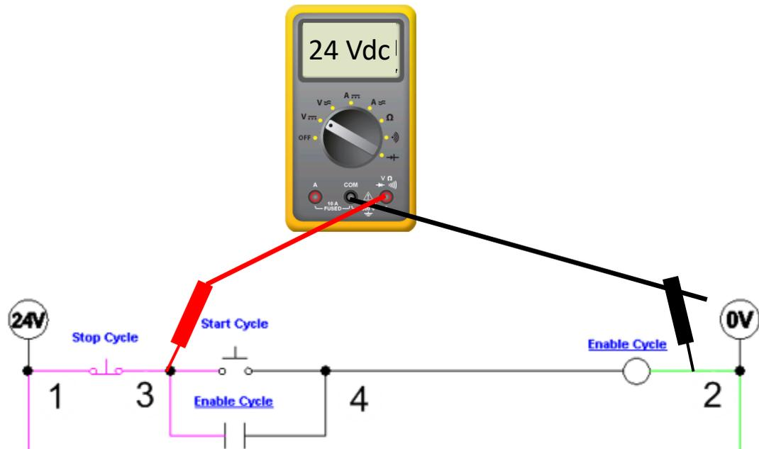
This slide shows what voltage will be measured across the 24Vdc power lines. It is 24Vdc, as shown in the top diagram. Notice that the dial has to be set for DC volts.
