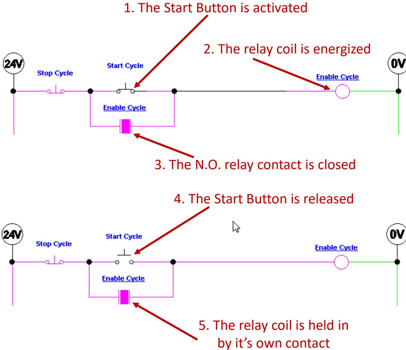
This slide shows the how a start/stop hold-in circuit works. The intent is that when the Start Cycle button is pressed, the Enable Cycle relay coil is energized, and when the Start Cycle button is released, the relay coil remains energized.
