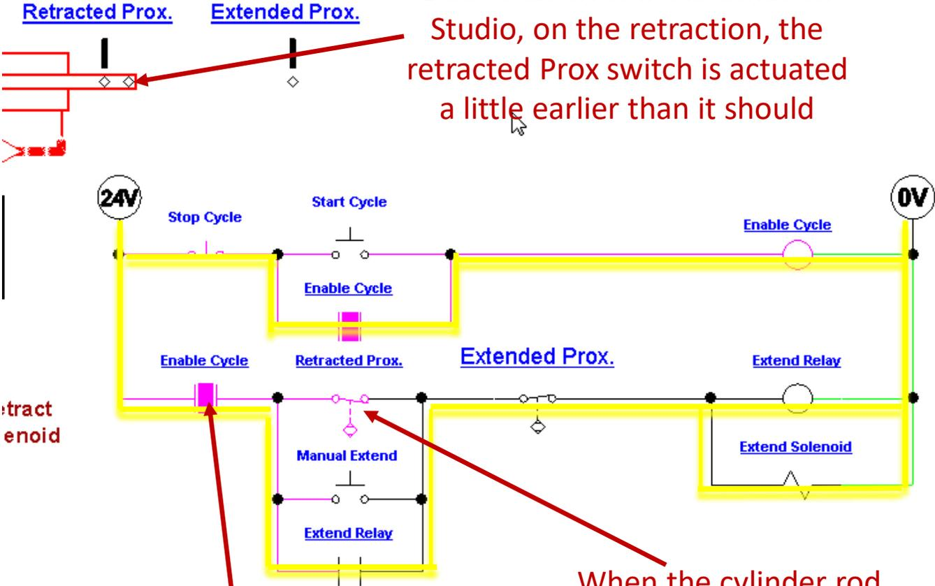
If a contact shows a purple block between the two contacts, the contact is passing power
