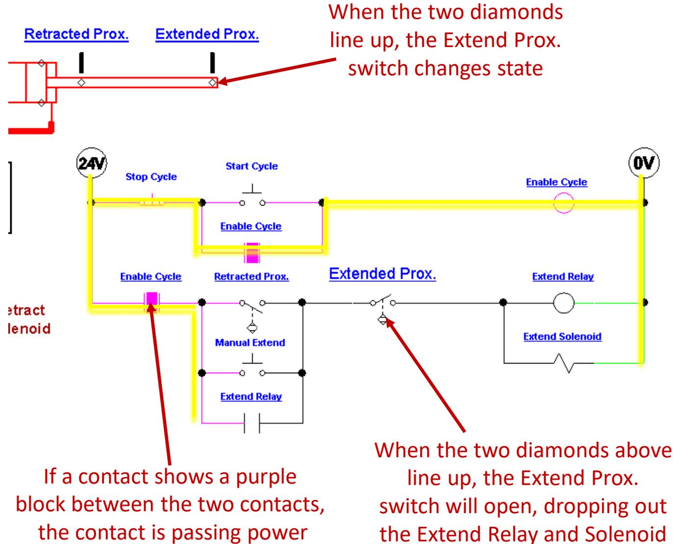
This graphic will give a further in depth explanation of the electrical circuit. This slide shows that the cylinder rod is fully extended, which actuated the Extend Prox switch. This will open the switch in the last rung of the electrical circuit, which will in turn drop out the Extend Relay and Extend Solenoid coils. This will cause the 5/2 valve to shift back to the default position (due to the spring return), which will start retracting the cylinder.
