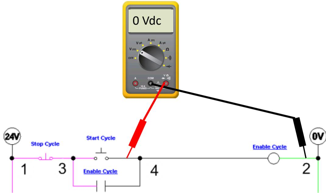
This slide shows that between nodes 4 and 2, there will be no voltage. This is due to the fact that neither the Start Cycle pushbutton, or the Enable Cycle relay are actuated.
