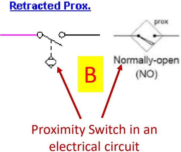
Proximity Switch in an electrical circuit
