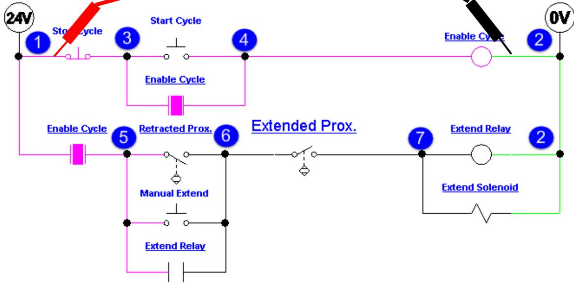
This slide will show the voltages that should be measured if the first rung is energized (Enable Cycle is pulled in), and the second rung does not have the relay and solenoid powered, due to the N.C. Extended Prox switch being actuated (between nodes 6 & 7).
