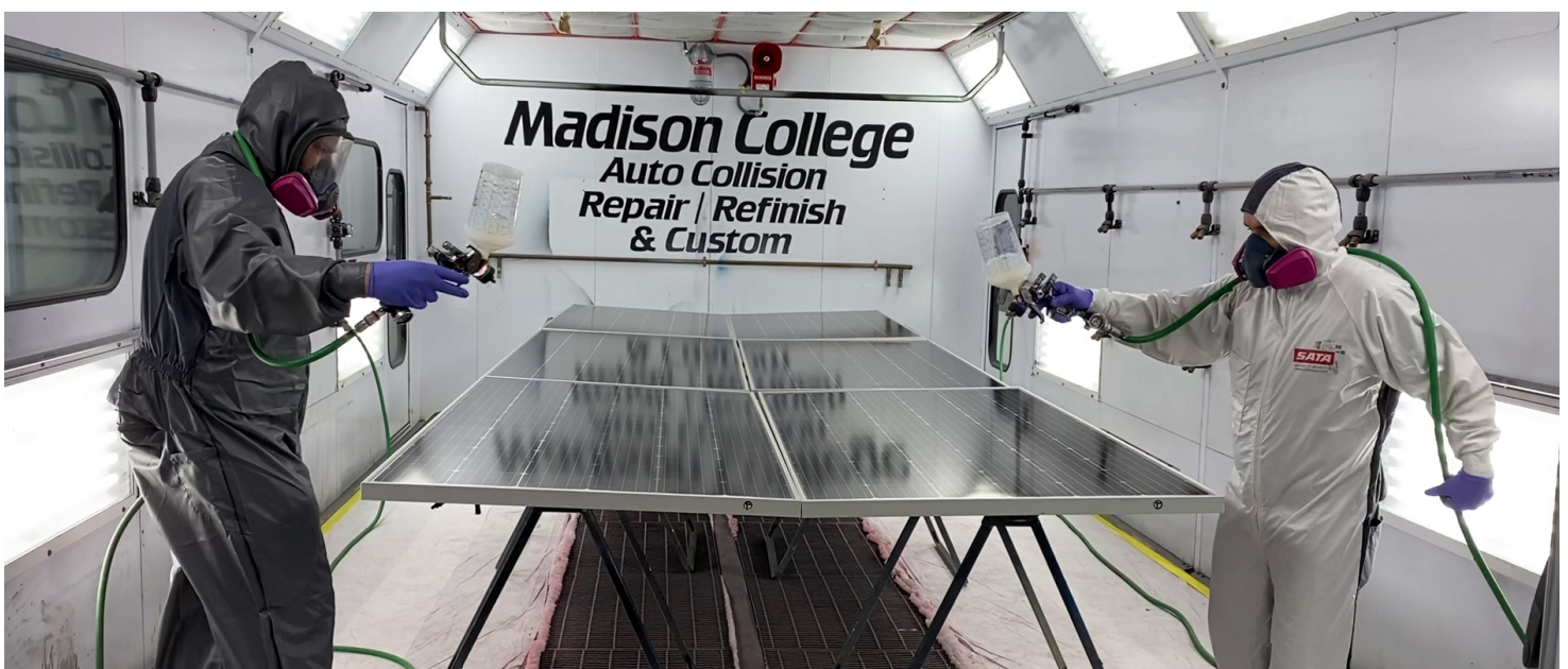
Madison College students spray deposit a nanoparticulate thin film coating to impart anti-soiling and self-cleaning properties to the surface of solar photovoltaic panels as part of an ongoing research and development project.
