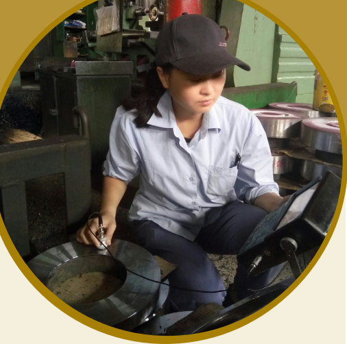
Technicians often use straight-beam ultrasounds to test raw materials for flaws prior to machining.
