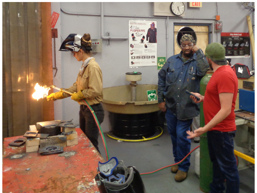
An instructor lights an oxyacetylene cutting torch at the 2021 AWS Instructor Institute.
