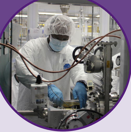
An Ivy Tech student loads a wafer into a sputter deposition tool to create a micro-pressure sensor during an SCME undergraduate research experience.
