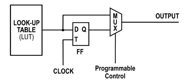
This figure shows a simplified and generic logic block (LB) used in most FPGAs. Instead of a PAL, the logic is implemented in a look-up table (LUT). A LUT is essentially a programmable memory like a PROM but with a SRAM storage element such as a flip flop (FF).
