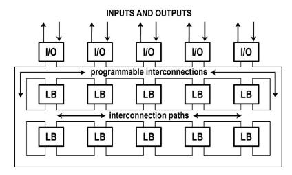
The physical architecture varies from manufacturer to manufacturer. In any case, the designer doesn't need to understand the interconnect scheme to use it to create a working design. The interconnecting paths may be row and column matrices or chains of multiplexers controlled by an SRAM or EEPROM or other programming element. In general, any I/O may be connected to any LB and any LB to any other LB.
