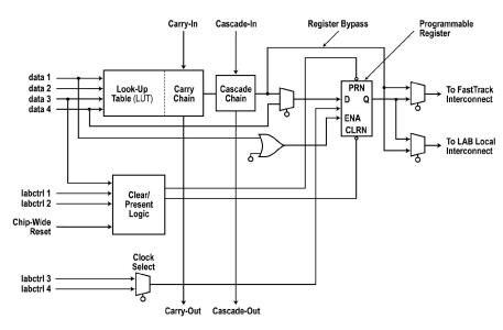
The logic element (LE) is the basic circuit for implementing random logic functions. A block diagram of a FLEX 10K LE is shown here. The basic logic functions are created with a 4-input LUT. The LUT contains carry in and carry out logic making arithmetic circuits easy to create. The LUT output goes to a cascade chain which provides interconnections to combine multiple LEs into larger circuits with more inputs and outputs.
