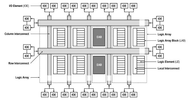
The EAB is a flexible block of SRAM cells with registers on the input and output. These cells can be used as RAM or a block of registers. Each EAB block contains 2048 bits which can be configured as 256 x 8, 512 x 4 1024 x 2 or 2048 x 1 SRAM.
