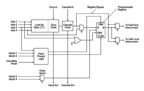
Each LE also provides a FF that can be configured as RS/latch, D, or JK type with programmable positive or negative-going clock and set/resets. Note the clear/preset logic available to the FF.
