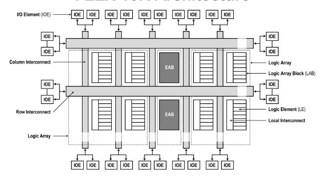
This figure shows a generalized block diagram of the FLEX 10K. It is make up of embedded array blocks (EABs), logic array blocks (LABs), and input/output elements (IOE) plus rows and columns of programmable interconnection paths. The local interconnect blocks allow programming within the EAB or LABs.
