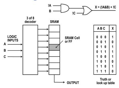
This figure illustrates the LUT concept with a 3-input LUT with eight storage locations. The 3 to 8 decoder is used to enable one of the eight SRAM cells. Each SRAM cell is a flip flop.
