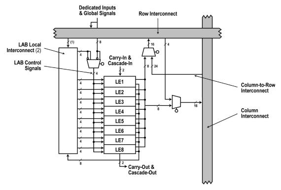
A variety of control signals are also present. The logic elements each have carry out and carry in lines to make arithmetic circuits easy to implement.
