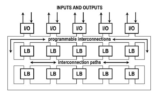
Like the CPLD, the FPGA consists of multiple logic blocks (LB) that can be interconnected to one another and to available I/O circuits with on-chip interconnect blocks. Here is one generic arrangement.
