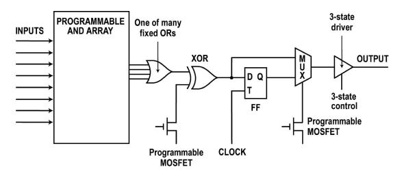
As an example, the OR output is fed to an XOR. If the XOR programmable input is binary 0, the XOR just repeats its input to the output. If the programmable input is binary 1, the XOR output is inverted.
