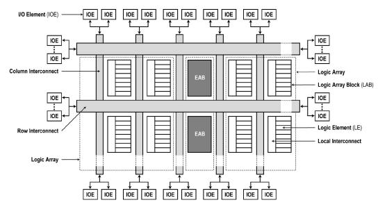
EABs may also be linked together to form even larger memories. There is a data input buffer register, a data output buffer register, and an address register. Remember that it takes an 11-bit address to identify 2048 RAM cells ( $2^{11} = 2048$ ).
