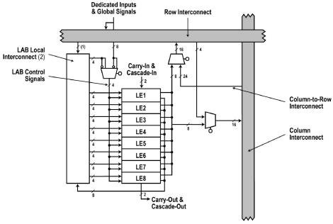
A logic array block (LAB) is made up of eight logic elements (LEs) and the supporting circuits. Multiple inputs are applied to the LEs from different sources and multiple outputs are developed. Local interconnects permit programmed connections within the block. The inputs and outputs connect to the row and column interconnect system through multiplexers.
