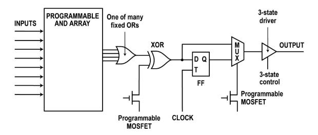
The logic block (LB) shown in the previous figures is a PAL with some interesting features. A generic example is given here. Remember that in a PAL, the AND array is programmable but the OR array is fixed. The fixed OR outputs are routed to other circuits that may or may not be used depending upon the programming.
