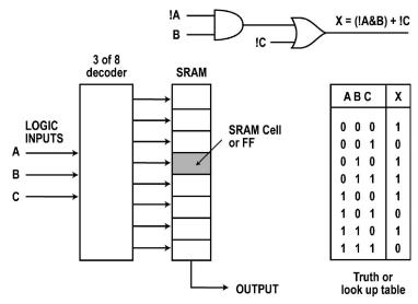
For instance, assume a logic operation expressed by the expression X = (!A & B) + !C. The equivalent logic diagram is also shown in the figure. The SRAM cells are programmed with a binary 1 or 0 corresponding to the output desired for each of the 3-bit input combinations.
