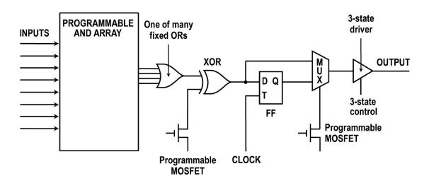
To bypass the FF, the MUX can be programmed to pass the FF input instead of its output. The output may be a three state driver. Logic blocks vary widely in terms of what circuits they contain and how they can be configured. Multiplexers are typically used to select one programming feature or another by programming.
