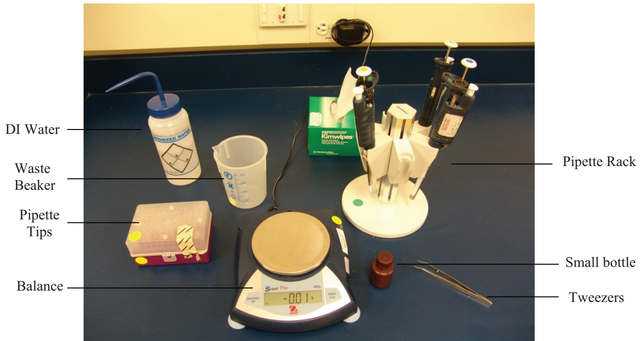
Figure 1: Pipetman® Verification Setup
