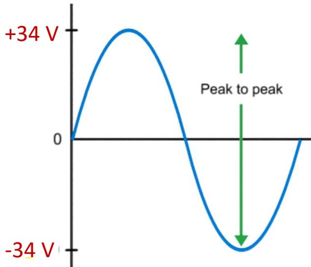
Continuing the AC quantity explanation, peak voltage is the highest point that the sine wave will go to. This value can be measured using an oscilloscope, or calculated from the measurement of the RMS value with the digital voltmeter measurement.
