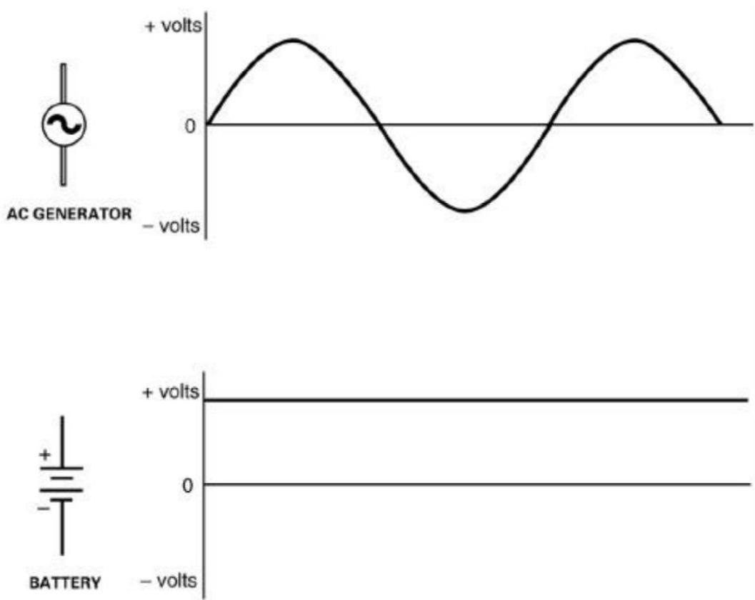
This slide compares the waveforms for both AC and DC power waveforms.
