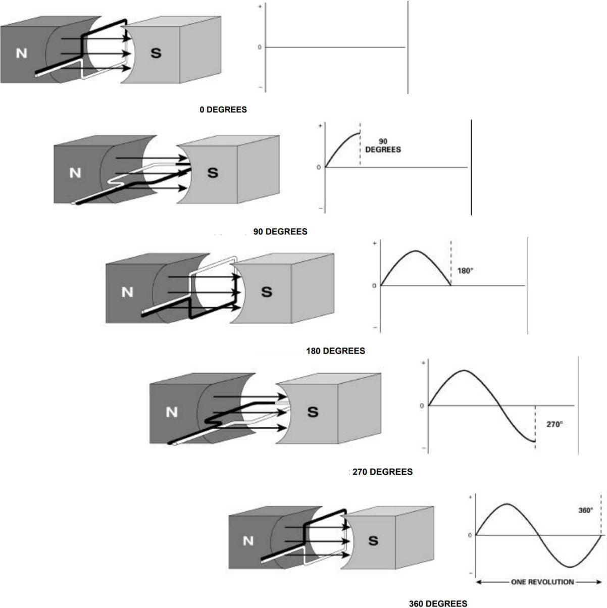
This slide shows how AC is generated, and the different quadrants of the sine wave.
