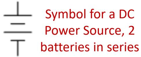
Symbol for a DC Power Source, 2 batteries in series
