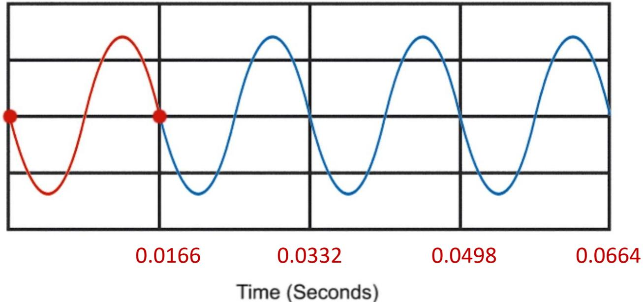
In the top graphic the sine wave in red is called one cycle. This cycle will occur in a specific time. Frequency of a sine wave defines the number of times that a sine wave repeats per second.
