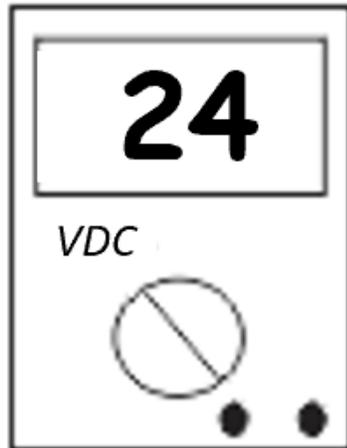
In this DC circuit, 24 Vdc is applied to a resistor. The important thing to understand is that current travels in only one direction. In DC circuits you may hear someone use the term electronic flow, which means that the current flows from the negative side of the DC power source to the positive side. Conventional current flow is positive to negative. This really doesn't matter. The important thing is that current is flowing in the circuit.
