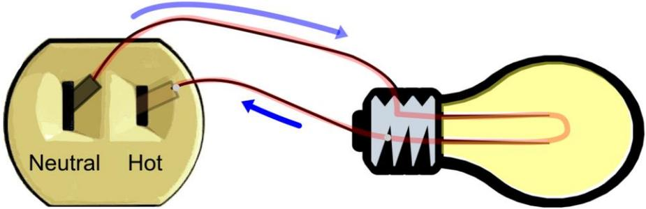
This is called the *positive alternation*, and the hot wire is positive with respect to the neutral terminal.
