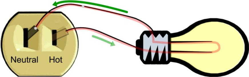
This is called the *negative alternation*, and the hot socket is negative with respect to the 0-volt neutral terminal.
