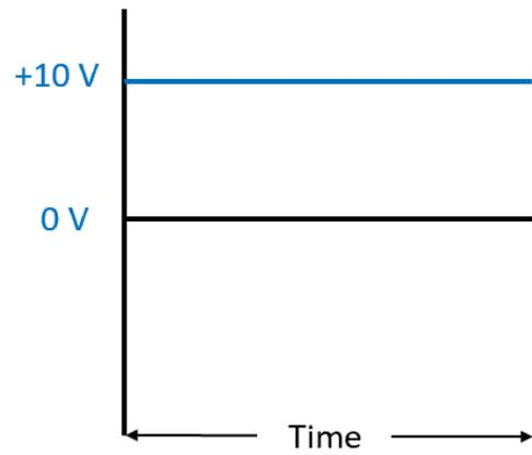
DC stays at a consistent voltage over time, and does not alternate or change direction
