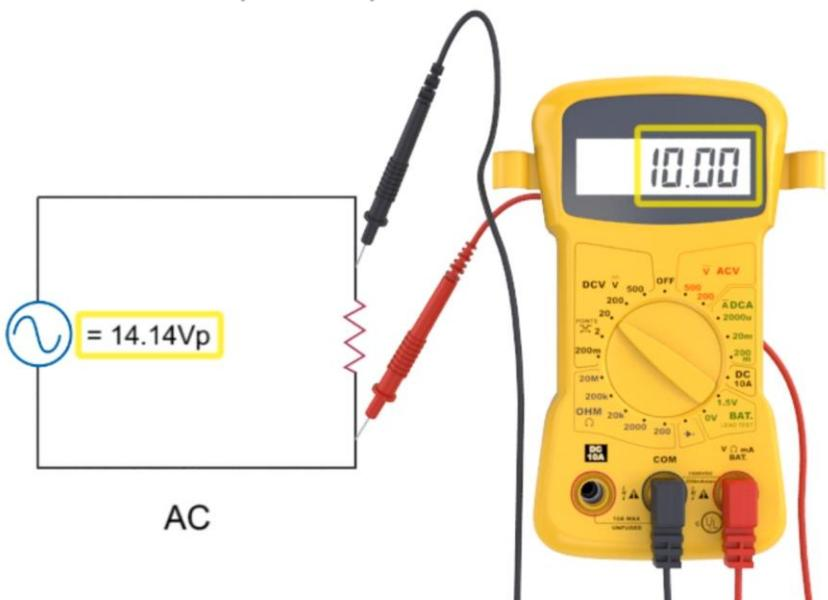
Three important terms to know when working with AC systems is Peak Voltage, Peak to Peak Voltage, and RMS voltage.
