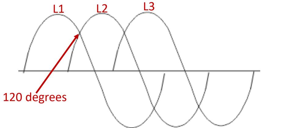
A three phase power waveform would look like this graphic. Notice that this is made up of three single phase waveforms. There is a 120 degrees phase shift with three phase. This means that 120 degrees into the first sine wave, the next single phase sine wave starts. Then 120 degrees later, the next sine wave starts.
