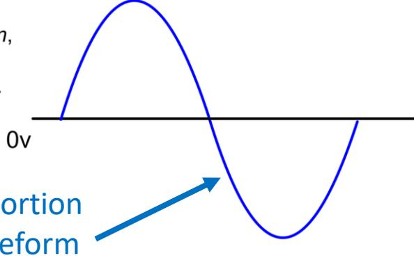
The current flows in the other direction on the negative portion of the AC sine wave, thus in the lower portion of the graphic, current flows from the Hot portion of the outlet, through the light, then back to the Neutral side of the outlet.
