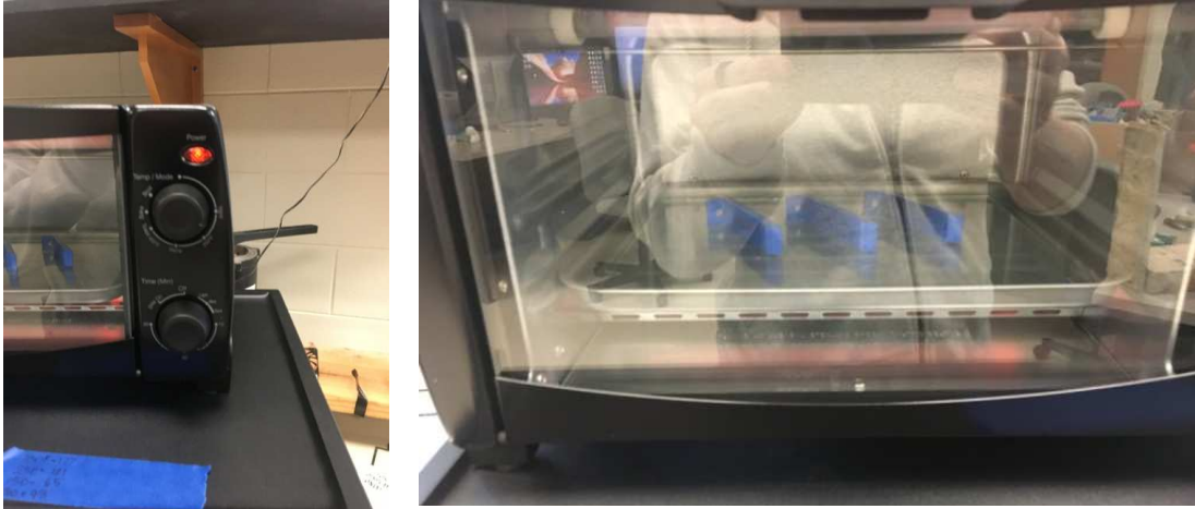
Figure 16: Example of test parts being annealed
