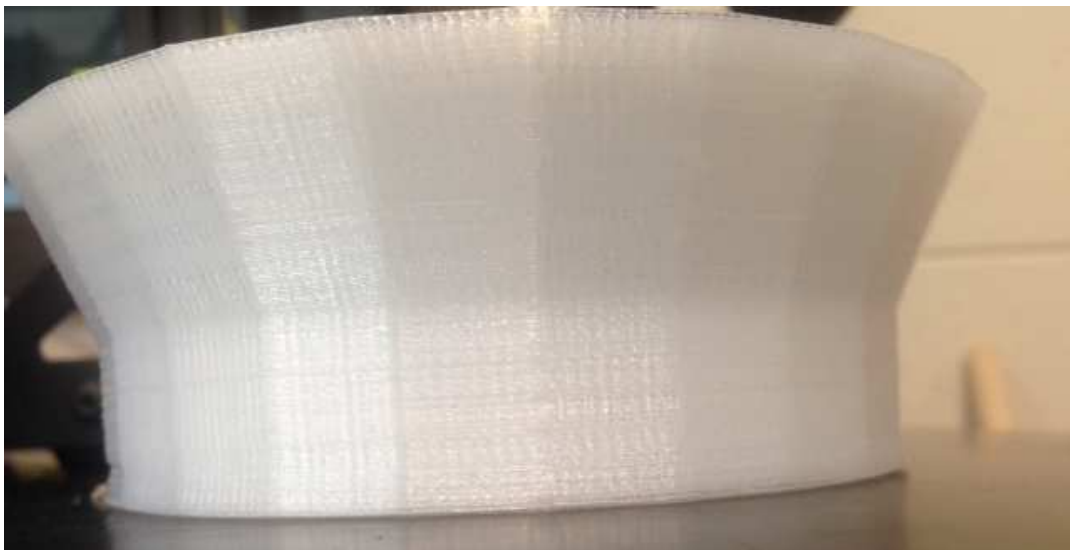
Figure 31: Test funnel showing angular-edged issue, due to original CAD model
