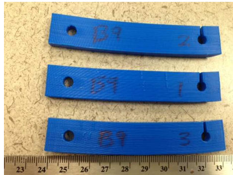
Figure 18: Picture of B9 parts curling after annealing
