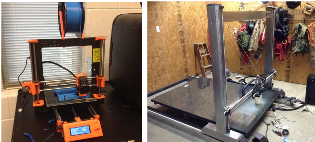
Figure 23: Pictures of Prusa I3 Mk2 (left) and custom large format FDM (right)
