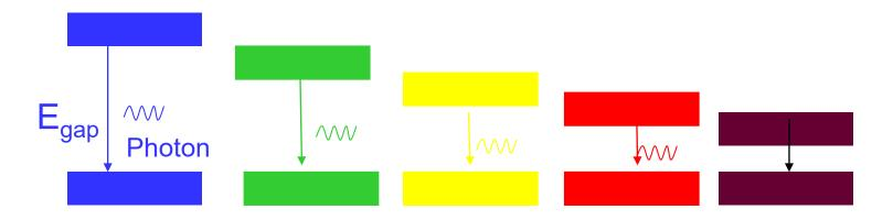
For an LED with a given band gap energy, illuminating photon has to be greater than this energy to excite a signal.
