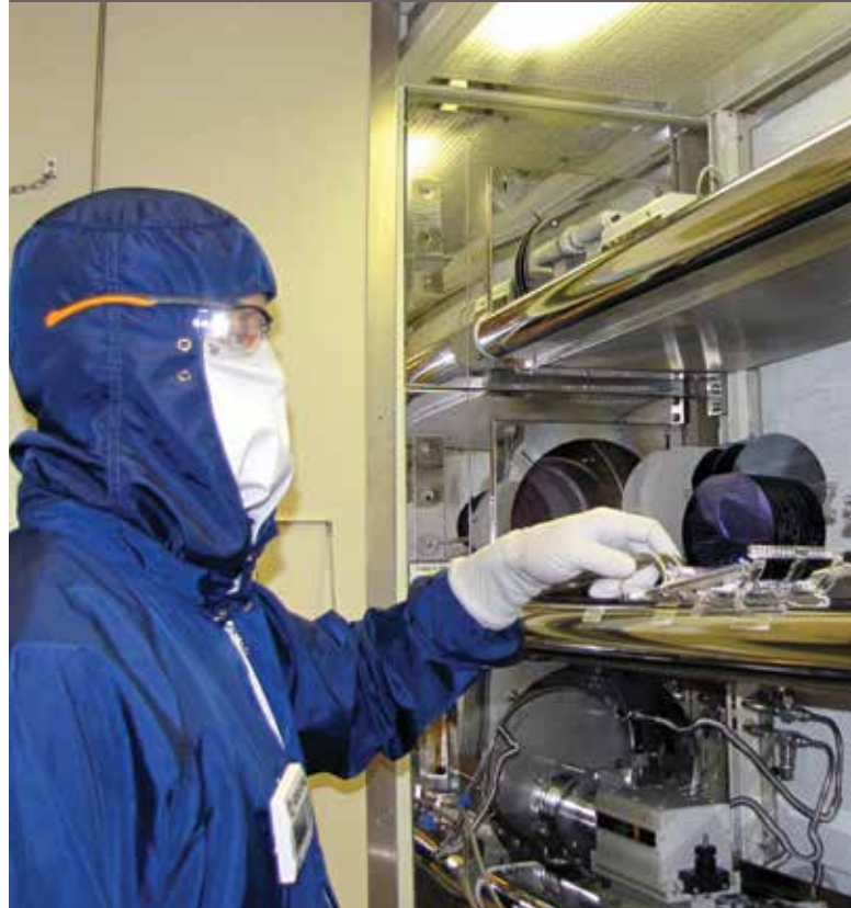
A Hudson Valley Community College graduate prepares silicon wafers for oxidation at GE Global Research.
