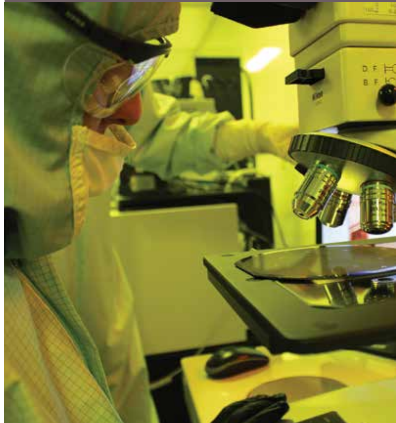
A technician inspects a MEMS wafer containing thousands of individual devices.
