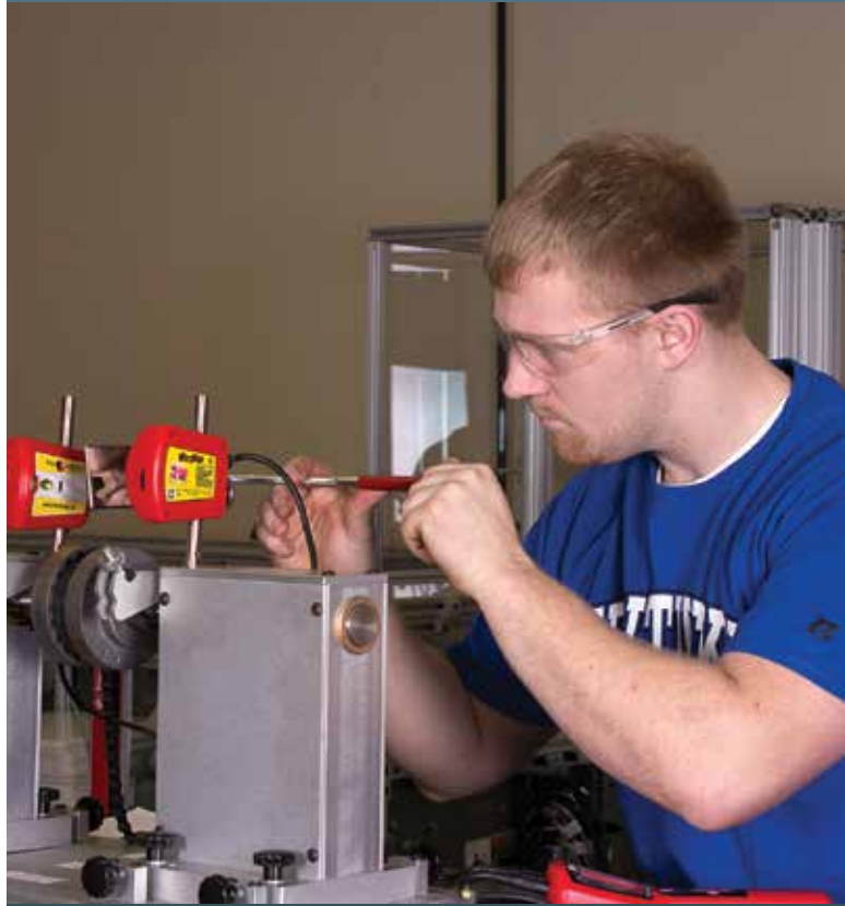
A technician checks the precision shaft alignment on a chain drive.
