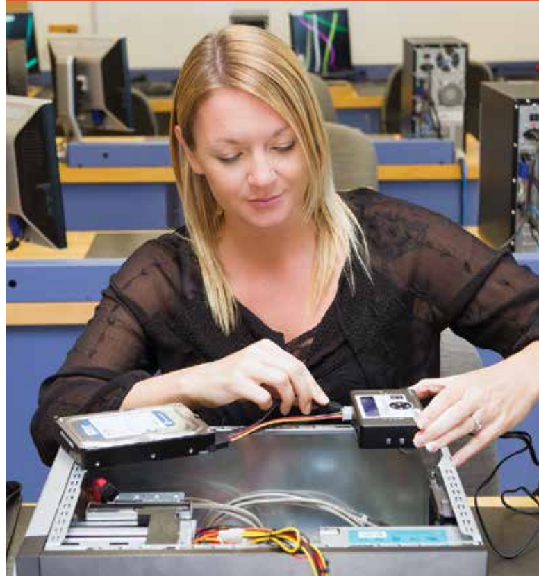
A technician uses a hardware write-blocker while creating a forensic copy of a hard drive.
