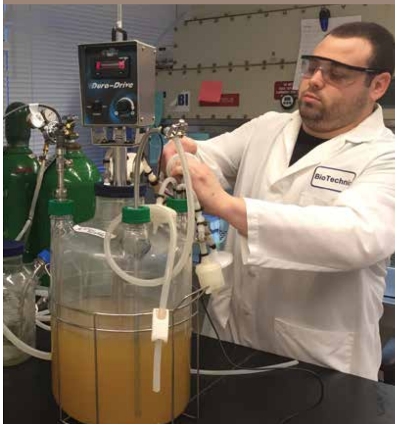
A technician adjusts a gas input line on a 20-liter bioreactor.
