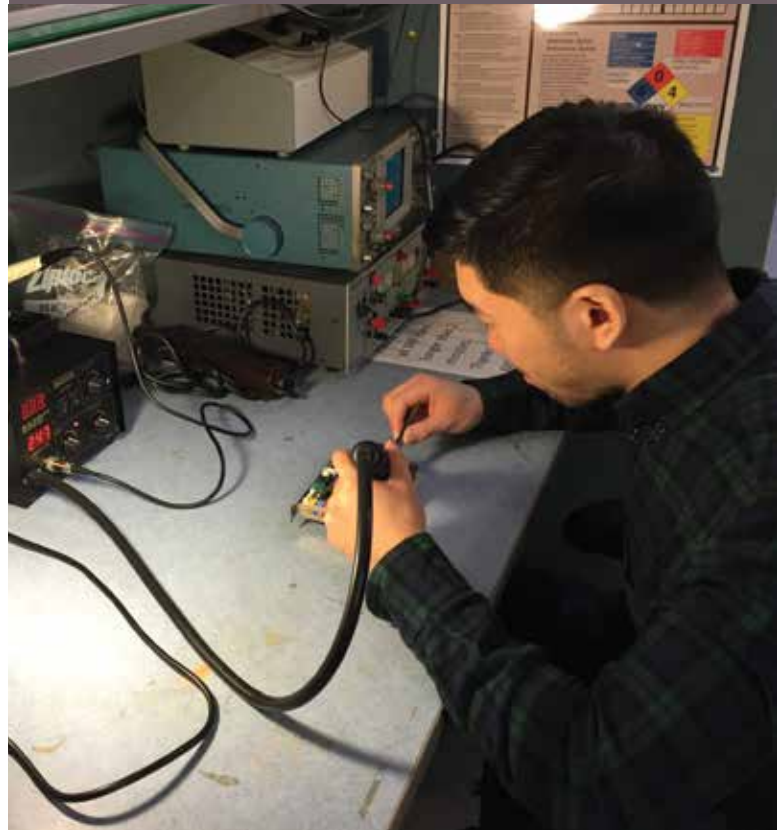
A nanotechnician disassembles a circuit board to analyze its heavy metal content using x-ray fluorescence spectroscopy.
