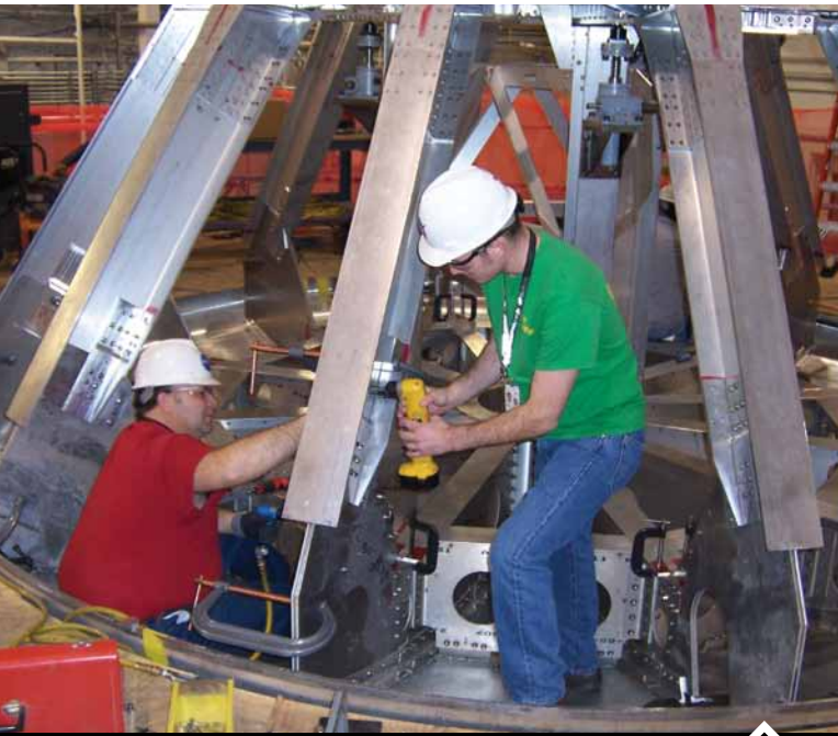
A CO-OPERATIVE STUDENT WORKS WITH A NASA TECHNICIAN ON THE FIRST FLIGHT TEST ARTICLE SIMULATOR OF THE ORION CREW EXPLORATION VEHICLE.
